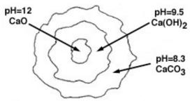
Diagram of a slag particle.
